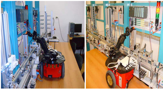
Figure 2. Flexible line for assembled/disassembled component
