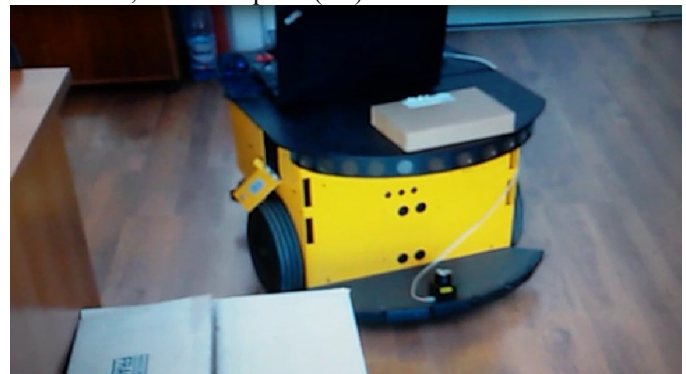
Figure 1. PoweBot avoiding an obstacle using Urg laser
