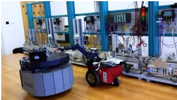
Figure 13. The two mobile robots loading reusable components in corresponding warehouse.
